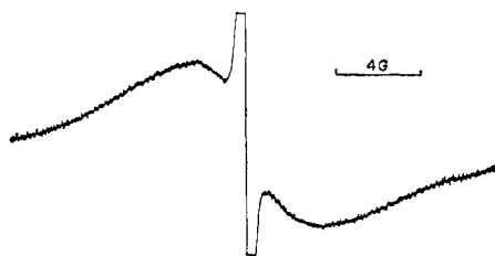
Figure 1. ESR first derivative spectrum obtained when naphthalene (1.4 M) was reduced with potassium in tetrahydrofuran. The clipped center peak indicates an off-scale reading.
